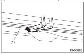
(2) Align the center claw of the cowl panel assembly to the cutout portion of the vehicle side, then install the cowl panel assembly.
